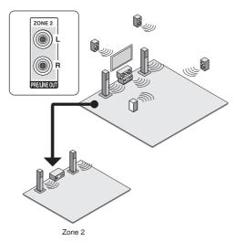
Volume can be adjusted with both the unit and the integrated amplifier used in a separate room. To adjust it with the unit, press RCV and then Home on the remote controller, select "Setup" - "7.Hardware Setup" - "Multi Zone" - "Zone 2 Out" and set the setting to "Variable". If you connect a power amplifier, be sure to make the setting and adjust the volume on this unit.
